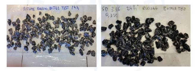
Figure 5e. Results Rolling Bottle Test inert basalt: on the left bitumen without additive, on the right bitumen with the addition of 0.3% of StarDope<sup>®</sup> 386 G.
