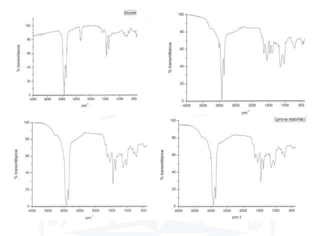
Figure 6I. Infrared spectrum acquired in transmittance by Fourier Transform Infrared Spectrometer in the frequency range between 4000 and 400 cm<sup>-1</sup>.
