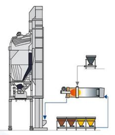
arrangement is required on the cylinder for introducing the RAP material and a dedicated feeding line consisting of a dosing hopper and a dedicated conveyor belt, recommending the use of the screen (note the fraction of milled material to be introduced), or directly in the final mixing phase without having to give up the use of the screen.
