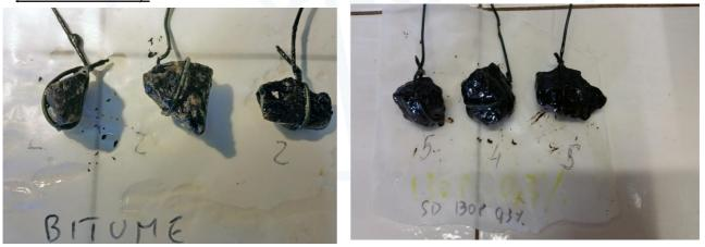
Figure 4i. Results Granitic inert tests: left bitumen without additive, on the right bitumen with the addition of 0.3% of StarDope<sup>®</sup> 130 P.
