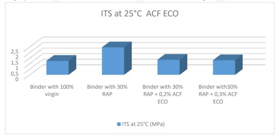
The graphs show the recorded values of Indirect Tensile Strength, performed at 25°C.
