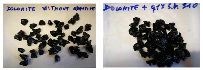
Figure 6c. Results Boiling Water Stripping Dolomites inert tests: left bitumen without additive, on the right bitumen with the addition of 0.1% of StarDope<sup>®</sup> 510.
