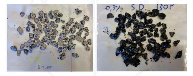
Figure 4a. Results Boiling Water Stripping Test basalt aggregates: left bitumen without additive, right bitumen with the addition of 0.3% StarDope<sup>®</sup> 130 P.
