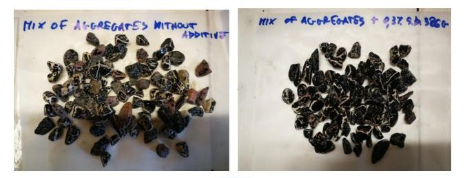
Figure 5h. Results Rolling Bottle Test aggregate mix: left bitumen without additive, on the right bitumen with the addition of 0.3% of StarDope<sup>®</sup> 386 G.
