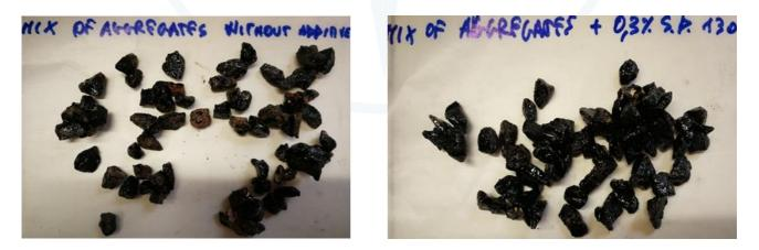
Figure 4d. Results Boiling Water Stripping Test aggregate mix: left bitumen without additive, right bitumen with the addition of 0.3% StarDope<sup>®</sup> 130 P.
