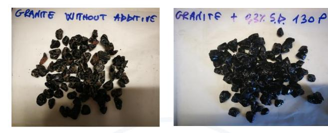
Figure 4f. Results Rolling Bottle Test inert granites: on the left bitumen without additive, on the right bitumen with the addition of 0.3% of StarDope<sup>®</sup> 130 P.
