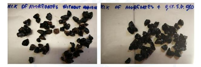
Figure 6d. Results Boiling Water Stripping Test aggregate mix: left bitumen without additive, right bitumen with the addition of 0.1% StarDope<sup>®</sup> 510.
