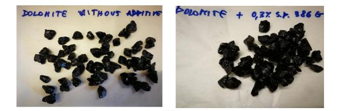
Figure 5b. Results Boiling water stripping Test inert granites: left bitumen without additive, on the right bitumen with the addition of 0.3% of StarDope<sup>®</sup> 386 G.
