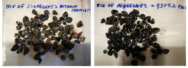
Figure 4h. Results Rolling Bottle Test aggregate mix: left bitumen without additive, right bitumen with the addition of 0.3% StarDope<sup>®</sup> 130 P.
