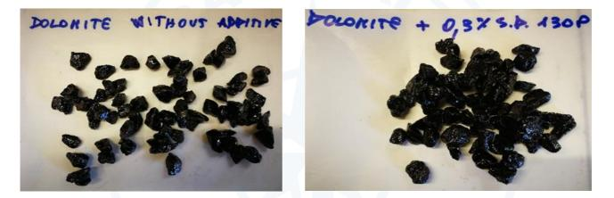
Figure 4c. Results Boiling Water Stripping Dolomites inert tests: left bitumen without additive, on the right bitumen with the addition of 0.3% of StarDope<sup>®</sup> 130 P.
