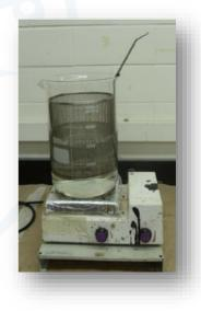
The first technique involves immersion in boiling water for a fixed period of time, evaluating visually, as a complete test, the degree of bitumen coating, expressed as a percentage. The covered surface, after 10 minutes of testing, must be typically over 80% in order to ensure a good durability of the mixture to the action of the water.
