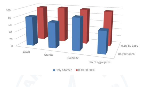
• Rolling Bottle Test Chart StarDope<sup>®</sup> 386G vs Non-Additive at t = 24h.
