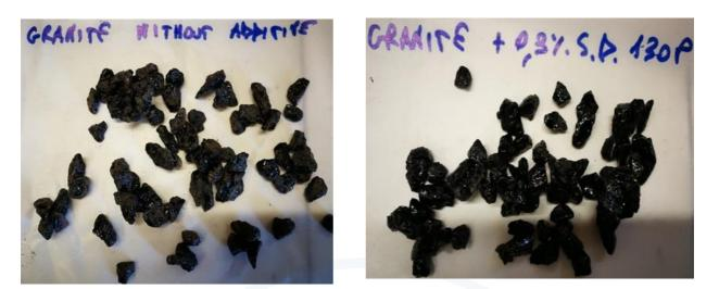
Figure 4b. Results Boiling Water Stripping Test inert granites: left bitumen without additive, right bitumen with the addition of 0.3% of StarDope<sup>®</sup> 130 P.
