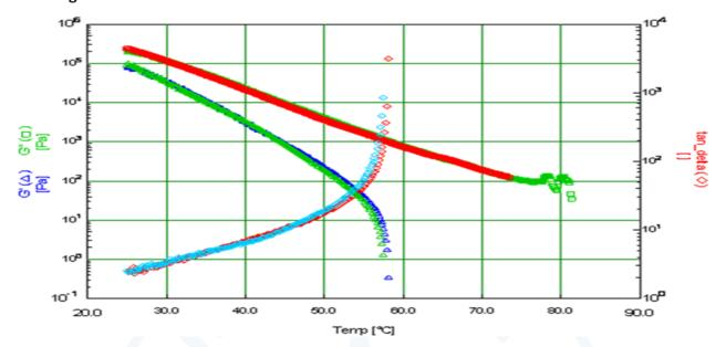
Graph 1. Storage module (G '') and loss module (G ') of a non-additive bitumen and of a bitumen additived with 0.5% of Warm-Mix<sup>®</sup> L. Department of Chemistry - UNIVERSITY OF CALABRIA -Arcavacata of Rende.
