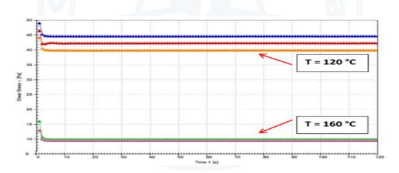
Graph 2. Overlap of "stress" curves of a sample of non-additive bitumen (blue curve), a sample of bitumen added with 0.5% of Warm-Mix<sup>®</sup> L (red curve) and a sample of bitumen admixed with 0.5% of StarDope<sup>®</sup> Warm-Mix 2G (orange curve) with deformation  $\gamma = 70\%$ , frequency  $\nu = 10$  Hz and temperature T=120°C and T=160°C.
