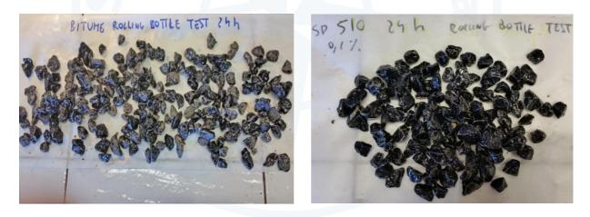
Figure 6e. Results Rolling Bottle Test inert basalt: on the left bitumen without additive, on the right bitumen with the addition of 0.1% of StarDope<sup>®</sup> 510.
