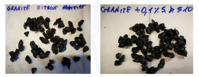
Figure 6b. Results Boiling Water Stripping Test inert granites: left bitumen without additive, on the right bitumen with the addition of 0.1% of StarDope<sup>®</sup> 510.
