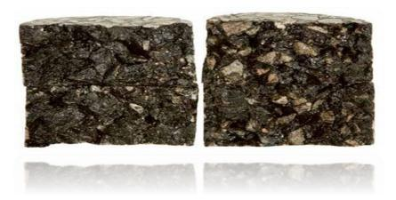
Fig. 3. Section of a sample: on the left, a section of the sample made with adhesion promoter, on the right a section of the sample made without adhesion promoter.
