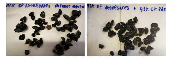
Figure 5d. Results Boiling water stripping Test aggregate mix: left bitumen without additive, on the right bitumen with the addition of 0.3% of StarDope<sup>®</sup> 386 G.
