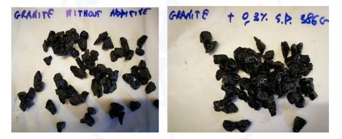
Figure 5b. Results Boiling water stripping Test inert granites: left bitumen without additive, on the right bitumen with the addition of 0.3% of StarDope<sup>®</sup> 386 G.
