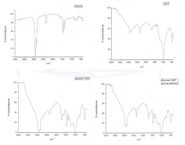
Figure 4I. Infrared spectrum acquired in transmittance by Fourier Transform Infrared Spectrometer in the frequency range between 4000 and 400 cm<sup>-1</sup>.
