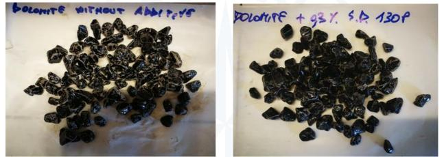
Figure 4g. Rolling Bottle Results Inert dolomitic tests: left bitumen without additive, on the right bitumen with the addition of 0.3% of StarDope<sup>®</sup> 130 P.
