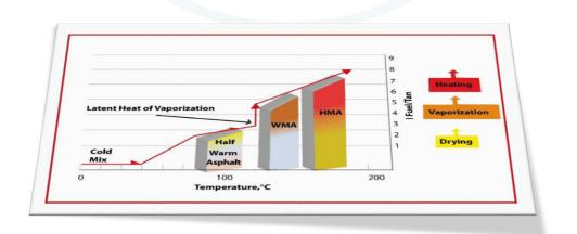
Fig. 1. Classification according to temperature range.
