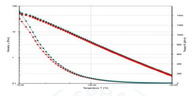
Graph 3. Overlap of curves of bitumen samples without additive and with 0.5% of Warm-Mix<sup>®</sup> L with shear rate = 0.5s-1 in a range of T=70-150°C.
