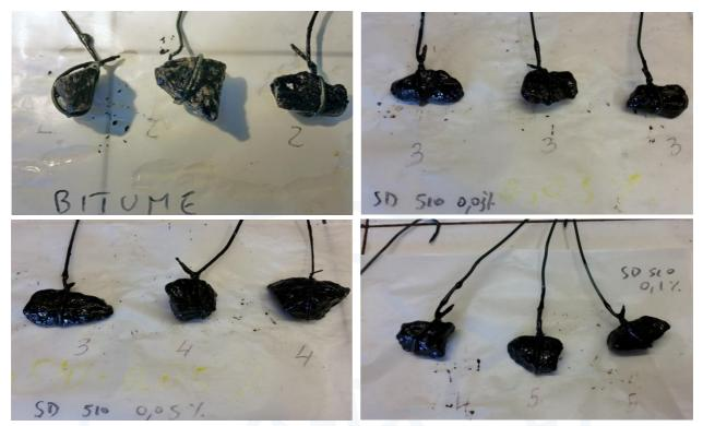
Figure 6i. Results Granitic inert tests: top left bitumen without additive, top right bitumen with the addition of 0.03% of StarDope<sup>®</sup> 510, lower left bitumen with the addition of 0.05% of StarDope<sup>®</sup> 510, in the lower right bitumen with the addition of 0.1% of StarDope<sup>®</sup> 510.
