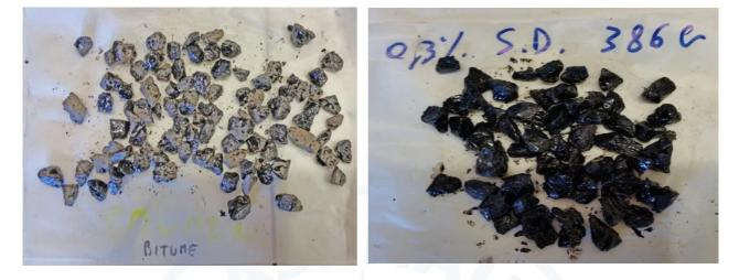
Figure 5a. Results Boiling water stripping Test basalt aggregates: left bitumen without additive, on the right bitumen with the addition of 0.3% of StarDope<sup>®</sup> 386 G.
