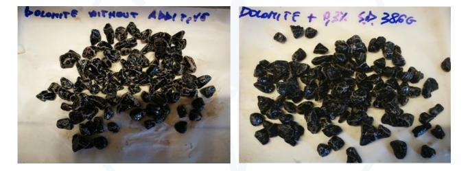
Figure 5g. Results Rolling Bottle Test inert dolomitics: left bitumen without additive, on the right bitumen with the addition of 0.3% of StarDope<sup>®</sup> 386 G.
