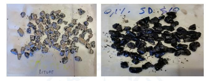
Figure 6a. Results Boiling Water Stripping Test basalt aggregates: left bitumen without additive, on the right bitumen with the addition of 0.1% of StarDope<sup>®</sup> 510.
