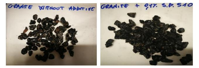
Figure 6f. Results Rolling Bottle Test inert granites: on the left bitumen without additive, on the right bitumen with the addition of 0.1% of StarDope<sup>®</sup> 510.
