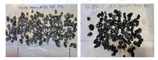
Figure 4e. Results Rolling Bottle Test inert basalt: on the left bitumen without additive, on the right bitumen with the addition of 0.3% of StarDope<sup>®</sup> 130 P.
