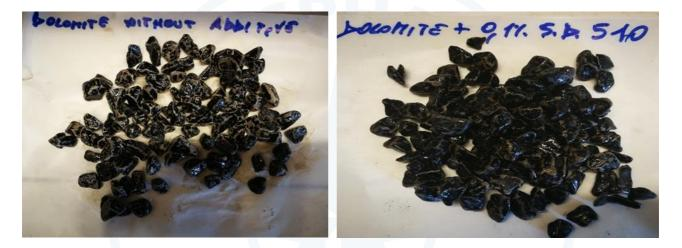
Figure 6g. Results Rolling Bottle Test inert dolomitic: left bitumen without additive, on the right bitumen with the addition of 0.1% of StarDope<sup>®</sup> 510.
