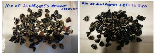
Figure 6h. Results Rolling Bottle Test inert mix: left bitumen without additive, on the right bitumen with the addition of 0.1% of StarDope<sup>®</sup> 510.
