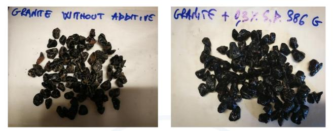
Figure 5f. Results Rolling Bottle Test inert granites: left bitumen without additive, on the right bitumen with the addition of 0.3% of StarDope<sup>®</sup> 386 G.
