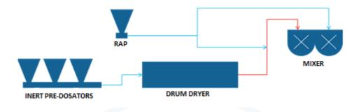
The choice of the addition mode substantially conditions the percentage of RAP material that can be used; in any way, it is mandatory that the final temperature of the mixture, coming out of the mixer, reaches at least 150°C. To this end, virgin aggregates must be overheated up to about 200÷250°C in addition to being dried.
