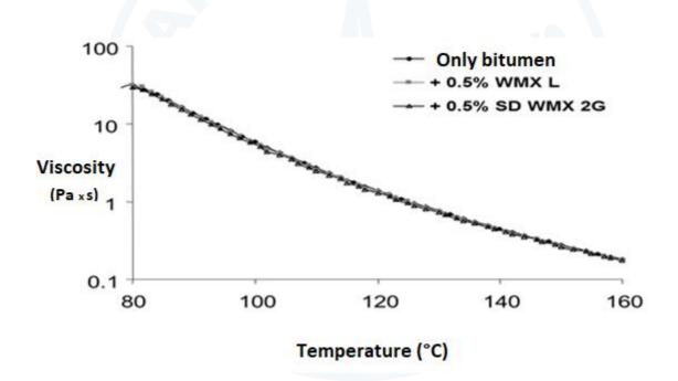
Graph 4. Trend of the viscosity as a function of the temperature of a sample of non-mixed bitumen, a sample of bitumen with 0.5% of Warm-Mix<sup>®</sup> L and a sample of bitumen added with 0.5% of StarDope<sup>®</sup> Warm-Mix 2G: as you can see, all the curves are superimposed, indicating that there is no change in the viscosity of the bitumen as these additives do not modify the physical properties of the bituminous binder.
